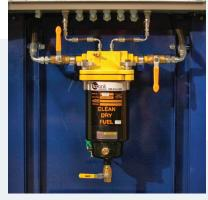
The integral fuel maintenance system allows for the use of existing fuel supply and return lines as the fuel supply pumps act as both the prime mover for the fill operation and the fuel maintenance cycles. This ensures clean fuel, regular exercise schedules for supply pumps and minimizes installation complexities.
