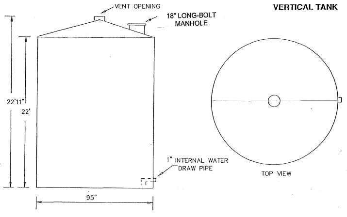
Weight \_\_\_\_5175 Bottom gauge \_\_\_\_6 Shell gauge \_\_\_\_6 Roof gauge \_\_\_\_10 NOTICE
