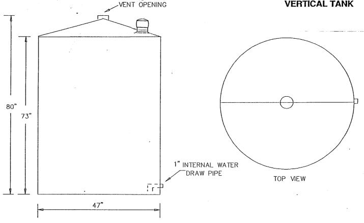
Weight \_\_\_\_535 Bottom gauge \_\_12 Shell gauge \_ 12 Roof gauge \_\_\_
