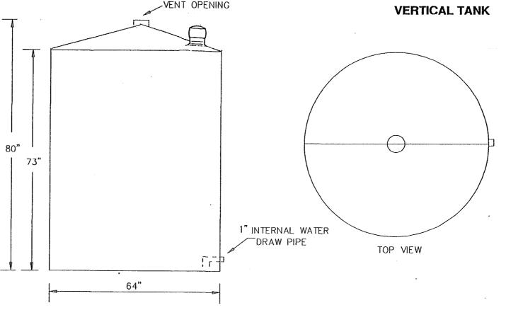
Weight \_\_\_\_875 Bottom gauge \_ 10 Shell gauge \_ 10 Roof gauge \_
