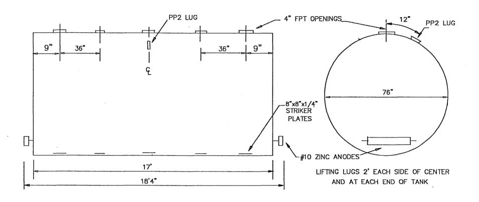
Weight 3,580 lbs. Shell Thickness 6 gauge Head Thickness 6 gauge
