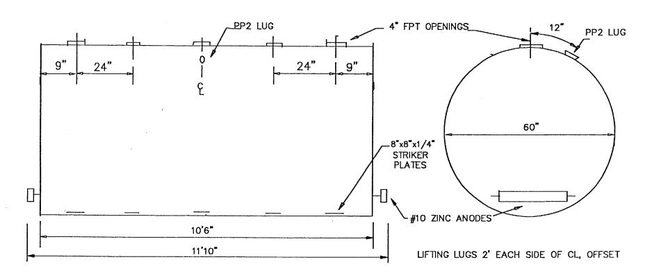
Weight 1,680 lbs. Shell Thickness 6 gauge Head Thickness 6 gauge
