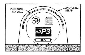
excavation sites exert significant buoyant forces on tanks. Buoyant forces are partially resisted by the weight of the tank, the backfill and the pavement atop the tank. Additional buoyant restraint, when required, shall be obtained by using properly designed hold-down straps in conjunction with concrete hold-down slabs or deadman anchors. The use of steel cable and/or round bar as hold-down straps on the tank is prohibited.
