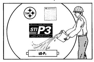
5.3 To assure immediate operation of cathodic protection system, each anode shall be thoroughly saturated with water at time of backfill operations.
