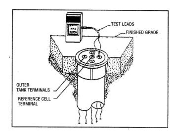
12.2 If the tank is connected to a PP4® test station the cathodic protection can be easily verified using a high impedance digital volt-meter. Touch the meter probes to the appropriate test head terminals as shown in the diagram above. As stated in 12.1, a minimum reading of -850 millivolts should be obtained.
