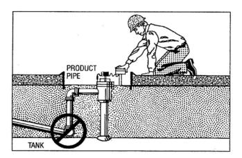
10.1 Contact between the steel tank and all other structures such as external and internal piping, pumps, valves, gauge and monitoring equipment, and grounding systems, will nullify the cathodic protection design. Prior to backfill, a simple continuity test between the tank lead wire and each
