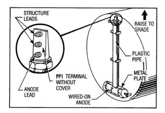
9.9 If the tank is equipped with a Protection Prover 1 (PP1®) monitoring system, which includes a monitoring test station mounted at the end of the tank, prior to any backfilling, extend the monitoring system to 4 inches (102 mm) below grade level without pulling it out of the mounting bracket. The PP1® test station shall be protected by a grade manhole of 7½ inches (191 mm) minimum diameter.
