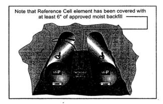
9.5 Locate the PP4® test head in its approximate final position and support with a wooden stake or other similar device. Connect the appropriate tank test wire from the reference cell element to the black test lead already installed on the tank using the hardware supplied or by performing a field splice.
