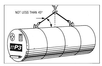
4.3 Tanks shall be carefully lifted and lowered by use of cables or chains of adequate length attached to the lifting lugs provided. A spreader bar shall be used where necessary. Under no circumstances shall chains or slings be used around the tank shell.
