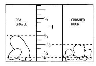
6.2 Special care shall be taken when installing backfill along the bottom sides of the tank to ensure that the tank is not damaged and is fully and evenly supported around the bottom quadrant.
