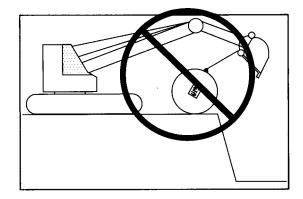
**3.1** Equipment to handle the tank shall be of adequate size to lift and lower the tank without dragging and dropping to prevent damage to the tank.
