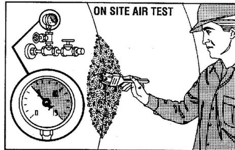
**3.2.3.3** With the tank depressurized, remove the test piping, temporary plugs, caps and seals. Reinstall the emergency relief vents, etc. which were removed in paragraph 3.2.1 above. Emergency vents are required on both the primary tank and the secondary tank.
